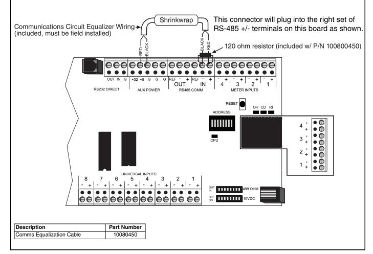
FIGURE 11: ROBERTS GORDON® ULTRAVAC™ Central Controller External Wiring
